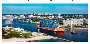
Recently, Port Everglades received three additional Super Post-Panamax container gantry cranes as we continue to make progress for larger cargo ships at our Port. The three 175-foot (53 meters) high Super Post-Panamax container gantry cranes, valued at \$15.1 million each, can handle containers stacked eight high on a ship's deck and reach 22 across. The new cranes
